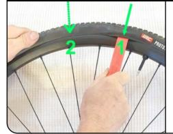
Place the tire lever next to the air valve and slide it between the tire and the rim. It's important to also press the tire with your hand to release it from the rim flank. This makes it easier to lift the tire out of the rim with the lever.
