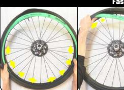
Put the PTN into the tire and slide it onto the rim bed.
